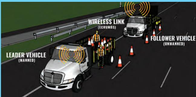
The Autonomous Impact Protection Vehicle will follow a manned maintenance vehicle (the leader vehicle). The lead vehicle transmits position, speed and direction to the impact protection vehicle so it can follow in the leader vehicle’s exact path. The impact protection vehicle will also carry radar obstacle detection systems to detect anything unusual in its path to avoid collisions.
